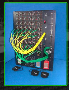
The 4 CPC sub-input channels are grouped 1-12, 13-24, 25-36, and 37-48. Channels 49-54 can be used as tie lines and have both male and female xlr connections in parallel providing convenience in patching for either inputs or returns. Ramlatch multi-pin outputs ensure a robust connection to the main, split 1 (monitor), and split 2 (recording) consoles This is a 15 rack space fully enclosed box.
